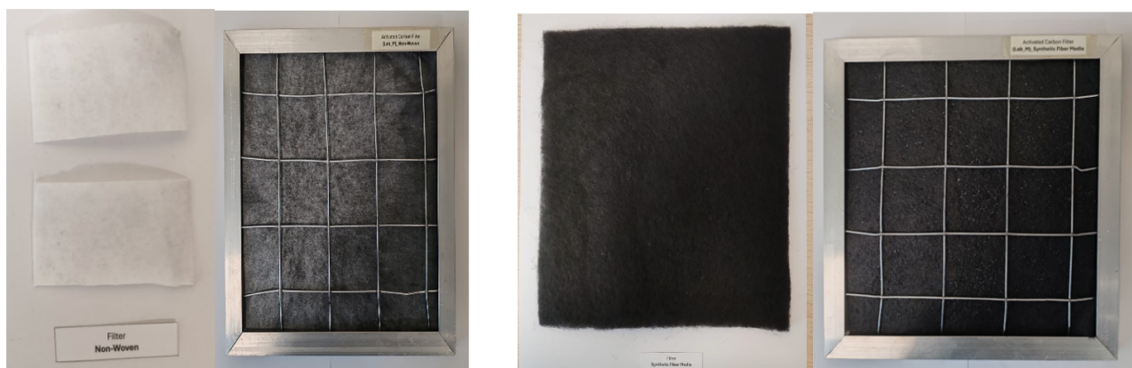
Fig. 4. (a) Non-woven PSAC filter before (left) and after (right) fabrication; (b) synthetic fibre PSAC filter before (left) and after (right) fabrication
