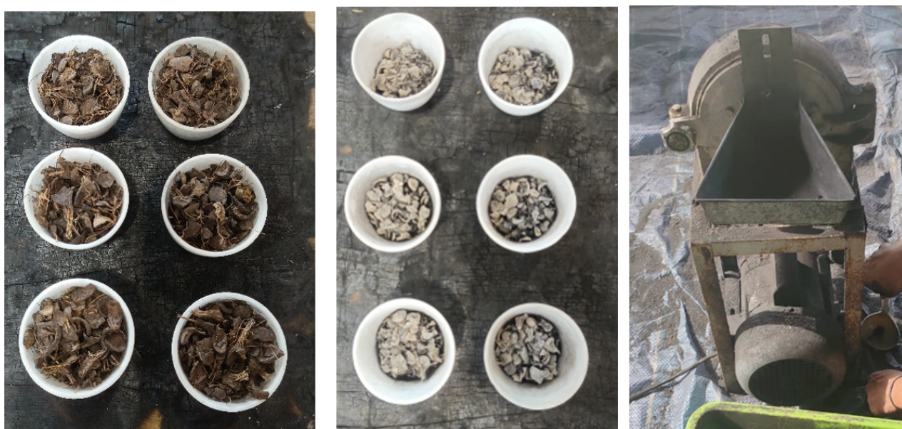
Fig. 1. Palm shells: (a) before carbonization; (b) after carbonization; (c) grinding machine
