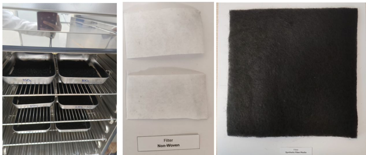
Fig. 3. (a) Palm shells being dried in an oven; (b) non-woven fabric material; (c) synthetic fibre fabric material
