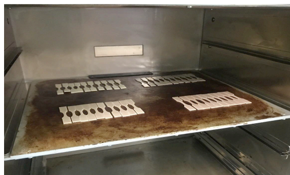
Fig. 1. Irradiation PVC sample placed evenly spaced inside the Memmert VO200 oven
