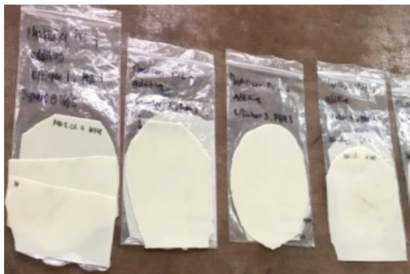
Fig. 5. Specimen after hot press were left for at least 24 hours in room temperature before further testing
