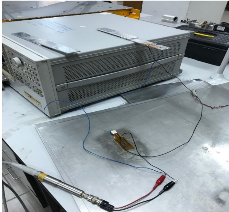
Fig. 3. Electromechanical Impedance Method (EMI) experiment setup
