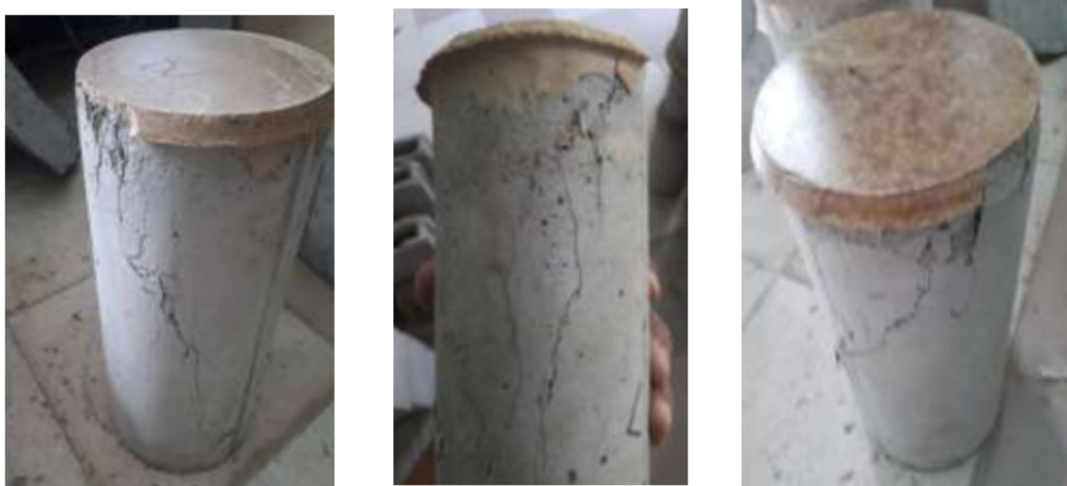
Fig. 2. Crack pattern of testing specimen
