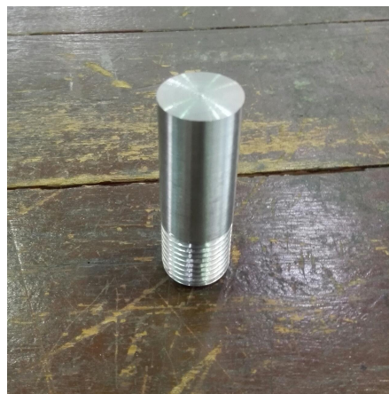
Fig. 5. Flat die for reshaping process
