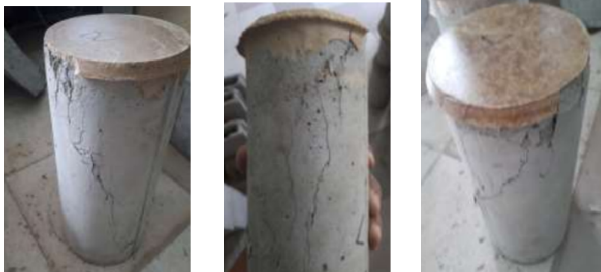
Fig. 2. Crack pattern of testing specimen
