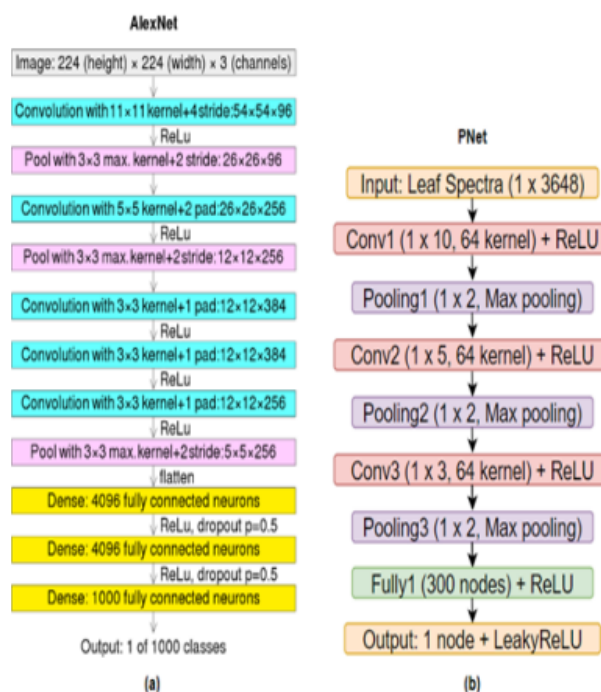
Fig. 2. (a) AlexNet Architecture (b) PNet Architecture
