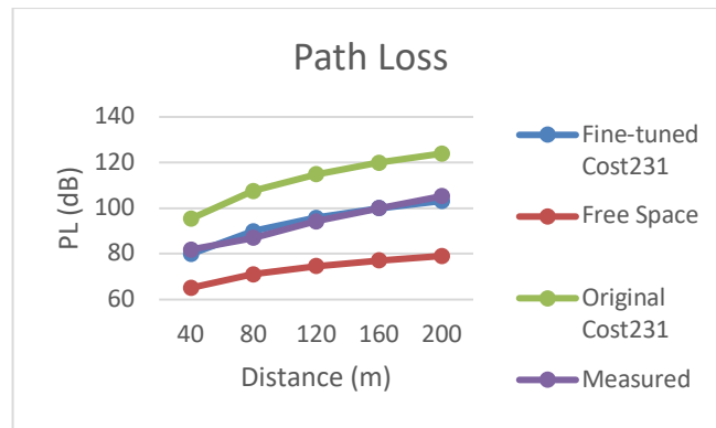
Fig. 3. Measured path loss, calculated and simulated path losses for Kampung Banyok
