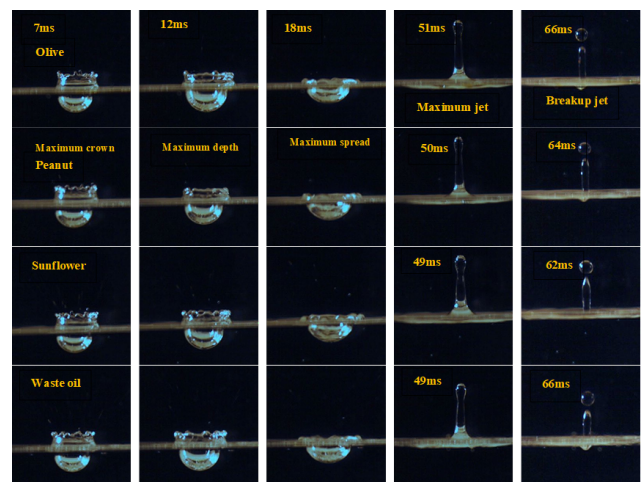
Fig. 9. Images oil droplet on distilled water pool under 80-degree temperature with V=3.96 m/s, We =986 olive, peanut 955, sunflower 972 and waste 1011 and D initial = (2.6 to 2.7)
