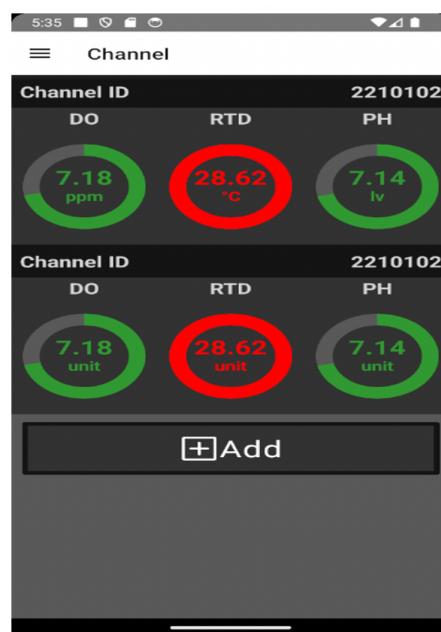
Fig. 9. Dashboard to monitor multiple water tank (channel)
