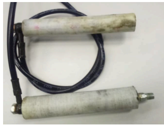
Fig. 8. a) The fabricated testing samples b) The testing hydraulic circuit that contains the pump (1), pressure gauge (2), the specimen pipe (3), pressure relief valve (4) and hydraulic tank (5)
