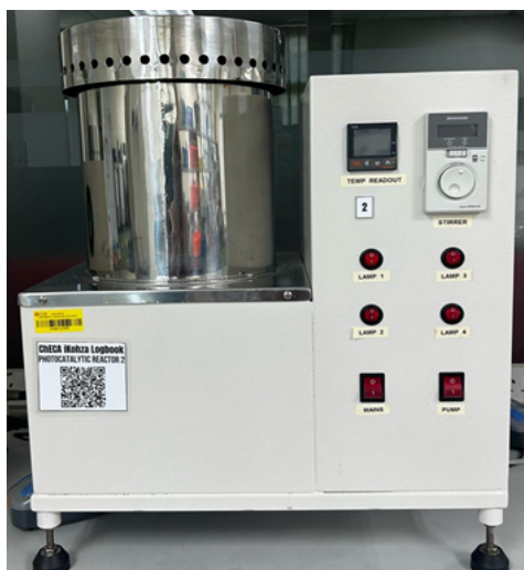
Fig. 2 Batch Flow Photocatalytic Reactor Diagram
