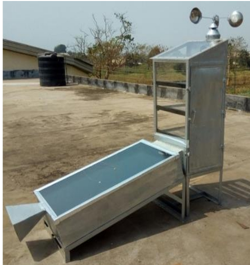
Fig. 7. Fabricated diagram of mixed mode passive solar stock fish dryer [9]
