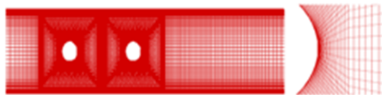
Fig. 2. Magnified view of a grid structure around the two tandem cylinders ( GR = 4 )
